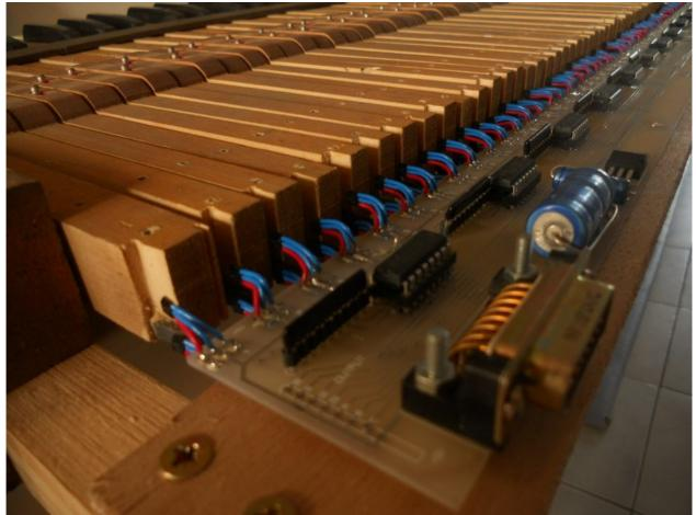
A complete keyboard needs 2 boards. Available with "on" contact or "on and off" sensor. Directly compatible with the KI\_7\_MIDI\_USB. Via a DB15 connector, as seen above.
