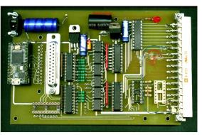
This parallel board can drive any real pipe organ, with resistor or inductive loads such as magnets or heavy duty magnets.
